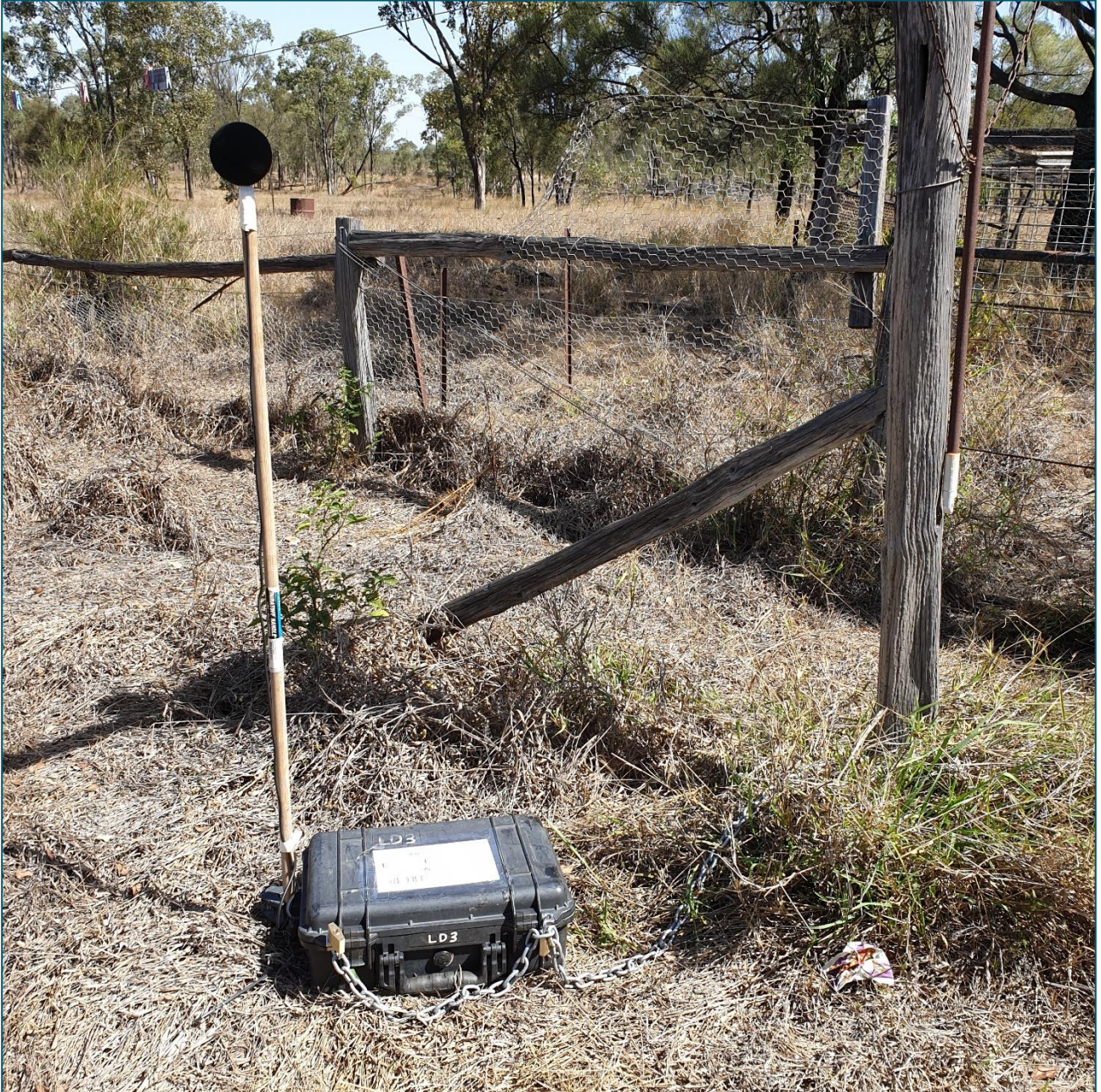
Figure B.1 Noise Logger setup at Receptor 6
