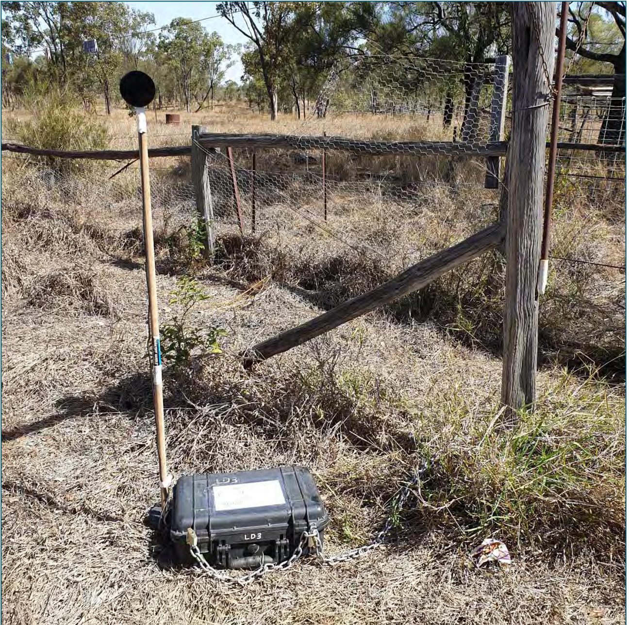
Figure B.1 Noise Logger setup at Receptor 6
