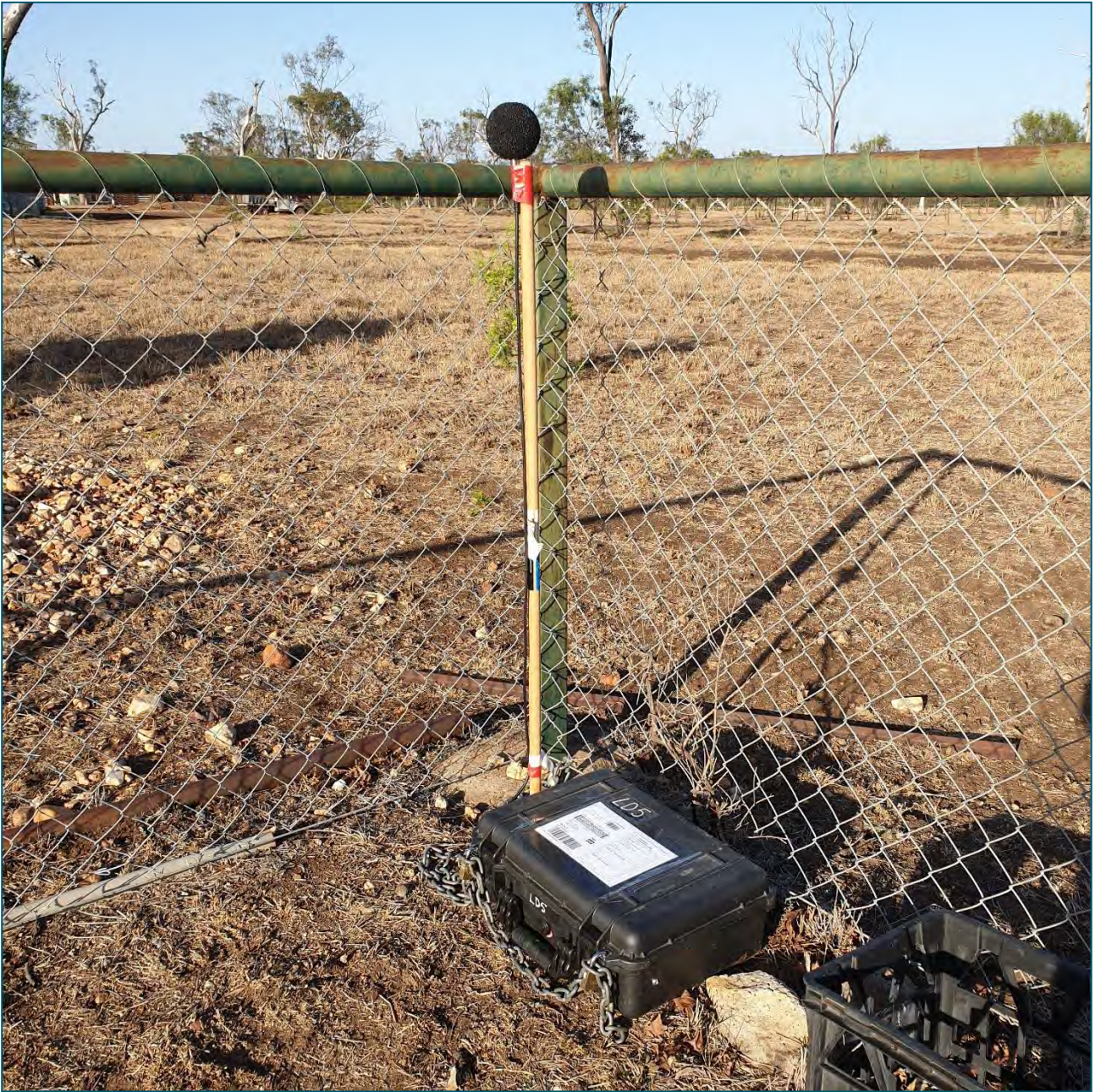
Figure B.2 Noise Logger setup at Receptor 8 (Luxor)
