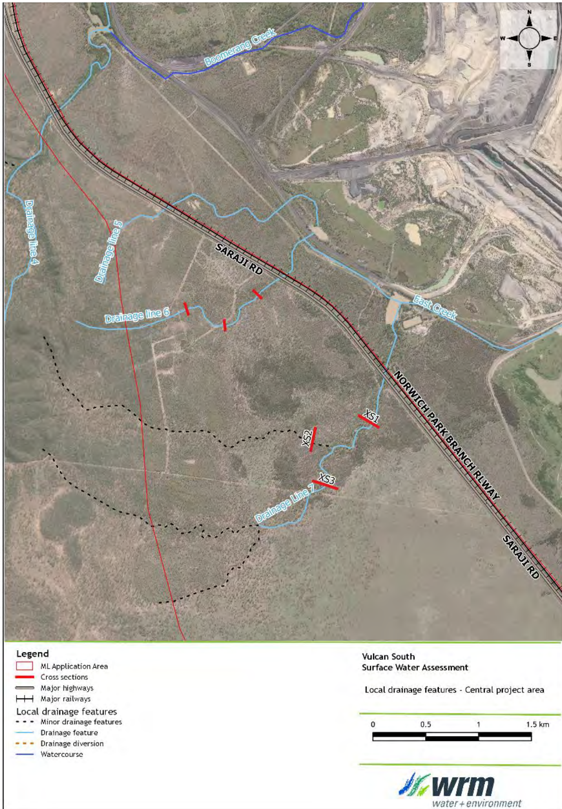
Figure 4.4 - Local drainage features - central Project area
