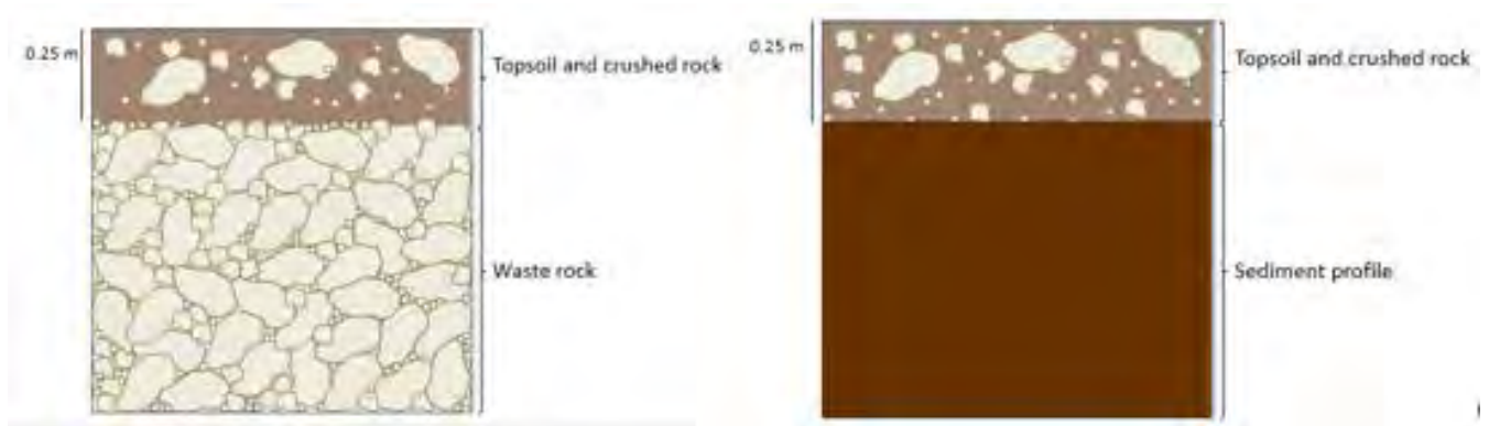
Figure 6-5 Highwall mining area cover design strategy for ex-pit WRD (left) and remaining areas (right)
