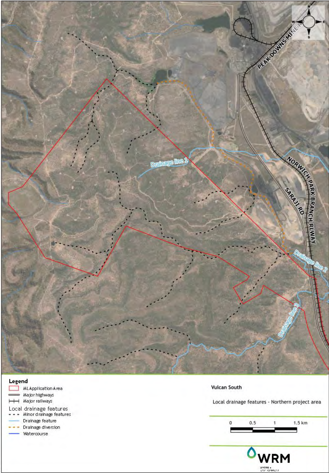
Figure 3.6 Local drainage features – northern project area
