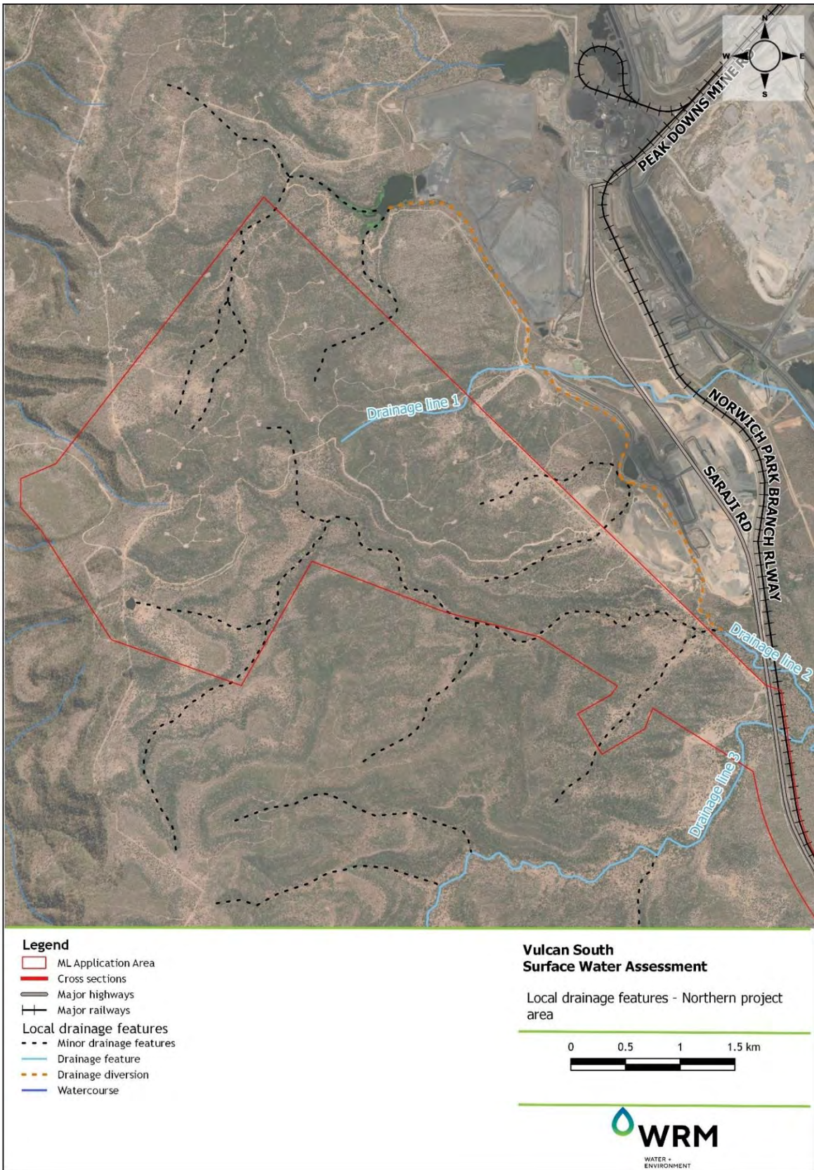
Figure 6-13 Local Drainage Features- Northern Project area
