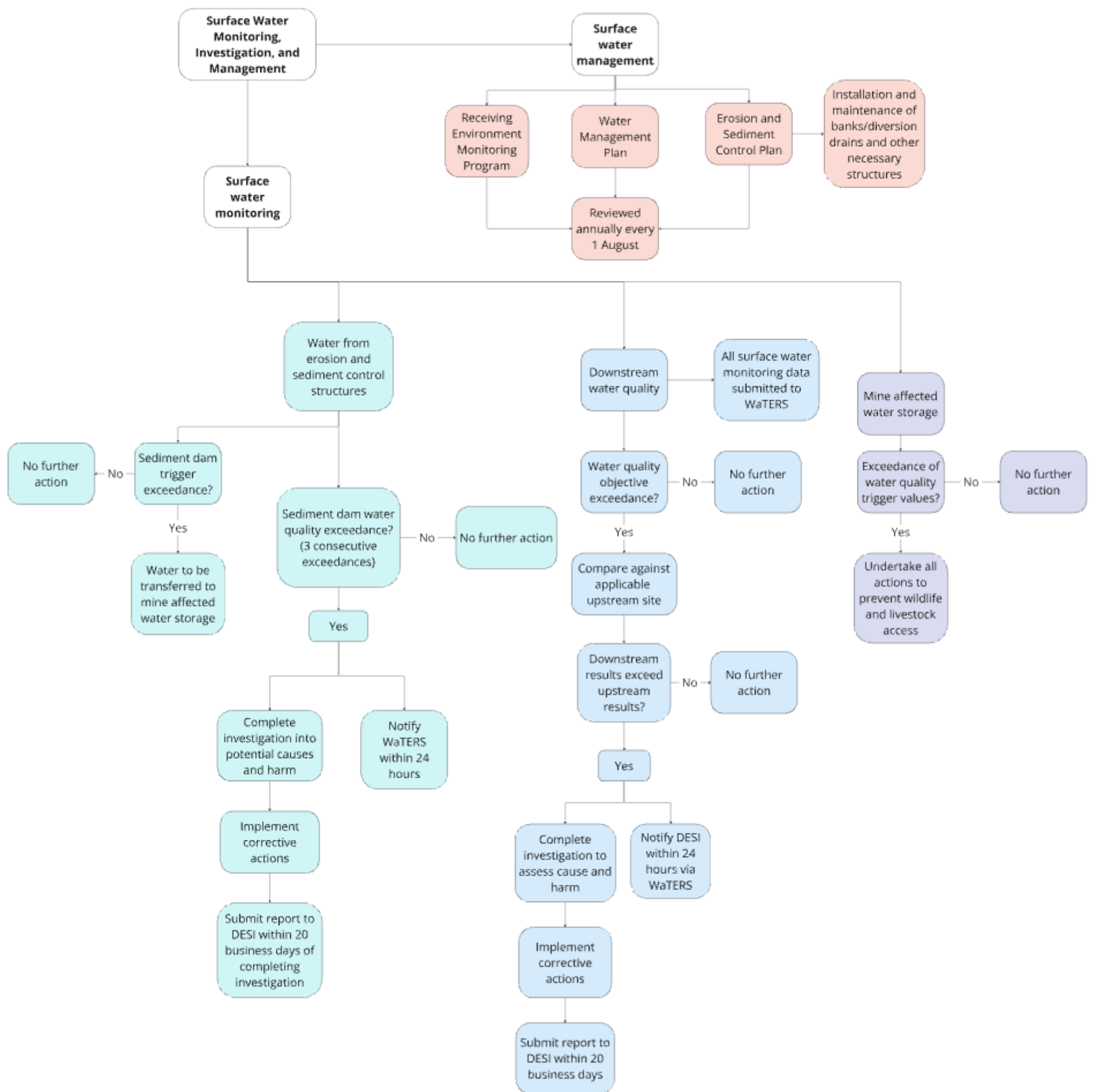
Figure 5.1 Surface water monitoring, investigation and management flowchart
