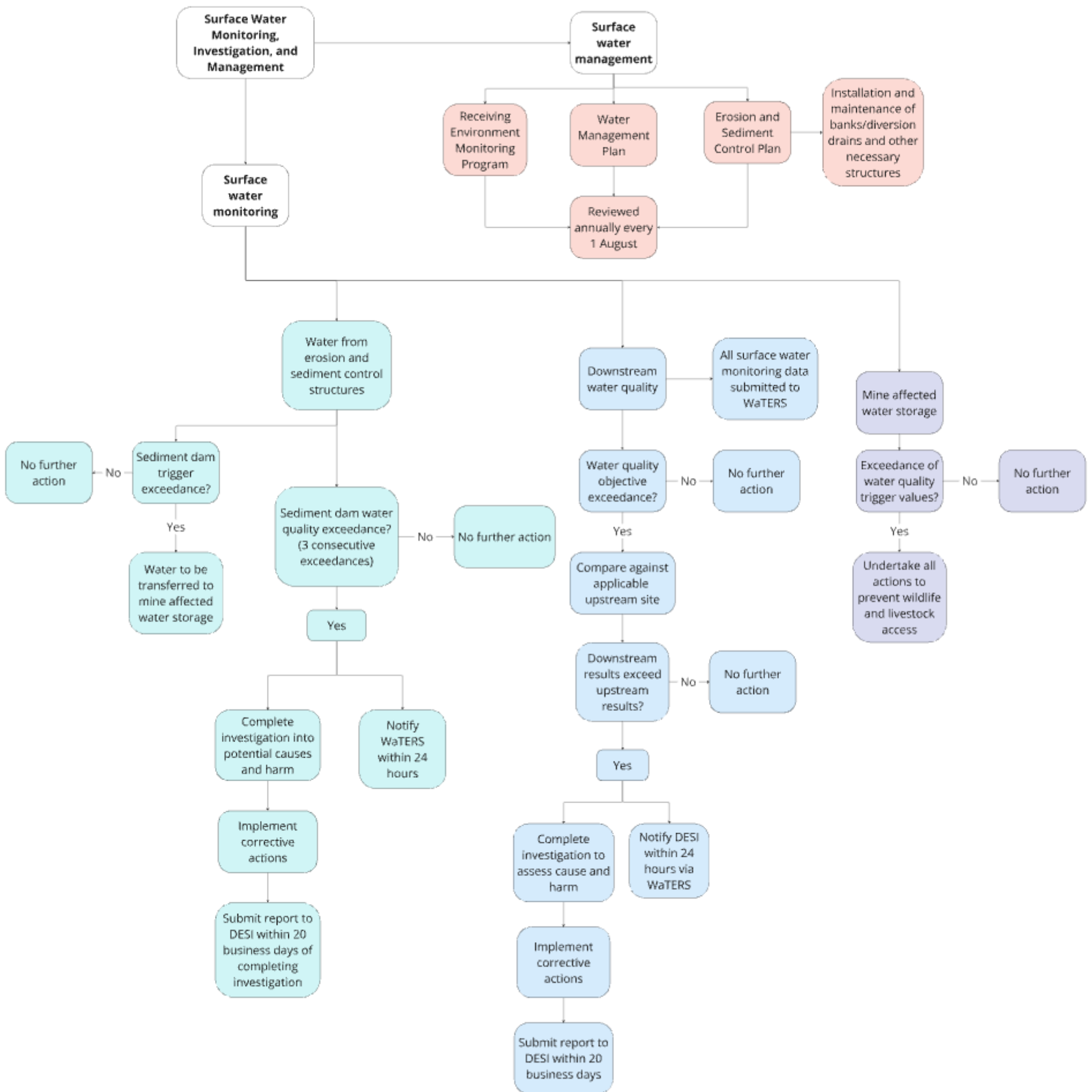
Figure 9.3 Surface water monitoring, investigation and management flowchart
